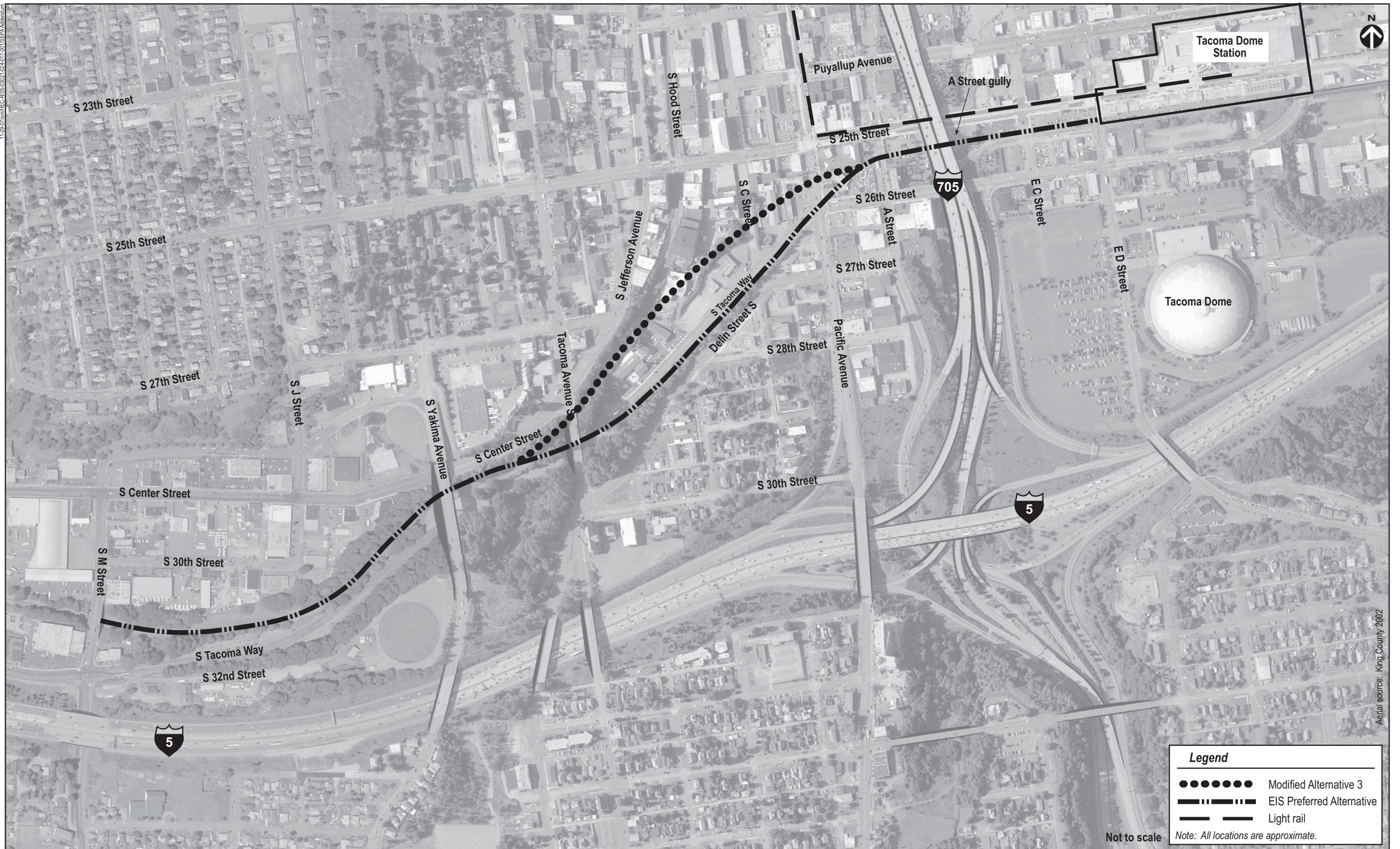
Exhibit B. Project alignment of the Tacoma section of the Lakewood-to-Tacoma Sounder commuter rail expansion under the EIS Preferred Alternative and Modified Alternative 3.
